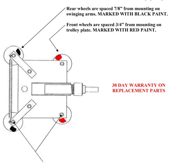
Enlarge mounting holes to 3/8" for new wheels with larger axles.
